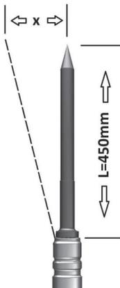
To check the degree of wear of the chisel bushing socket, insert the correct end of a new tool with a length of 450 mm into the chisel bushing socket!
