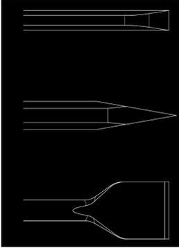
**Flat-tipped narrow chisel:** For demolishing and breaking apart hard materials (concrete)
