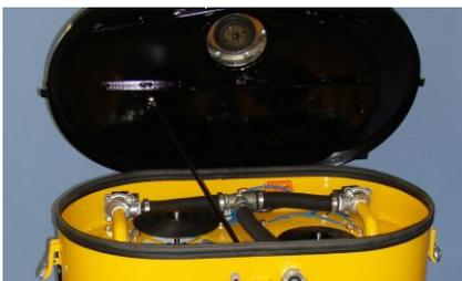
Easy access of filters and air valves by opening the top, the clean side of the dust collector.
