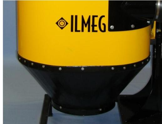
The X-Series filters are conical, specially designed for tough rock drilling applications. The conical shape supports the cleaning function in an excellent way. The filter material is made from water resistant material for long life.
