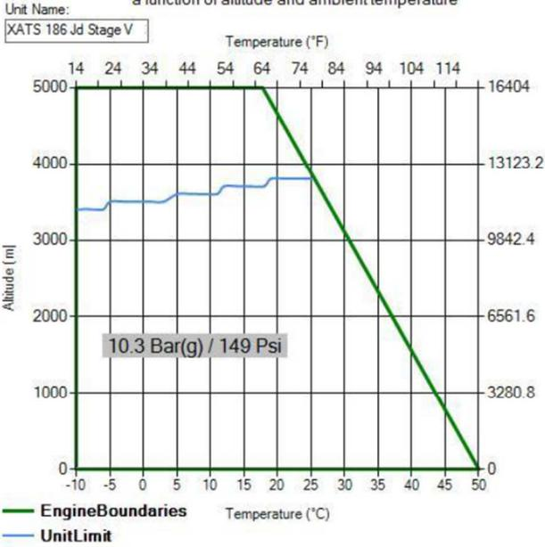
Graph represents working conditions, for starting conditions pls contact your Atlas Copco contact
