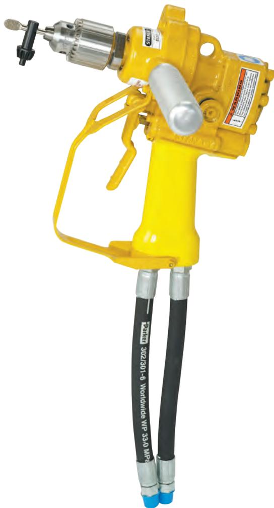
The Stanley **DL07** hydraulic drill is a forward/reverse, variable speed drill with a ½" keyed chuck for underwater drilling applications. The **DL07** has more than enough torque to drill most steel, masonry, wood or coral. A two position assist handle and trigger guard are standard. See chart below for speeds at select gpm of hydraulic flow. Painted hi-visibility yellow.
